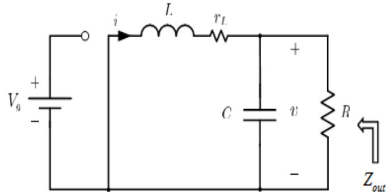
$$Z_{out} = (sL + r_L) \parallel \frac{1}{sC} \parallel R$$
