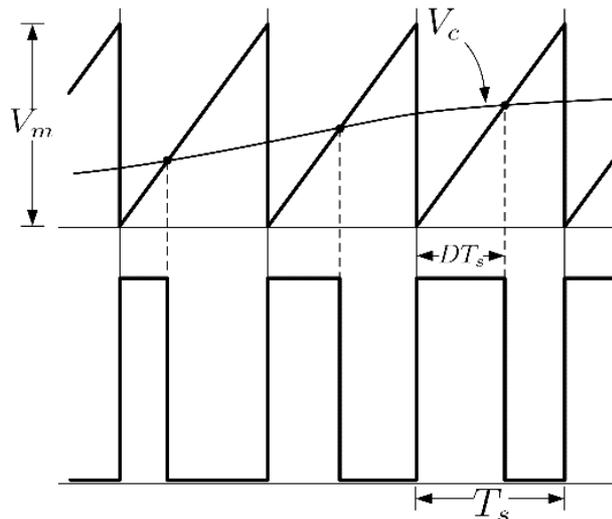
Sawtooth waveform has a peak-to-peak amplitude of  $V_M$ .
